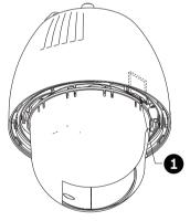
AUTODOME 7000 – Slot for SD card
