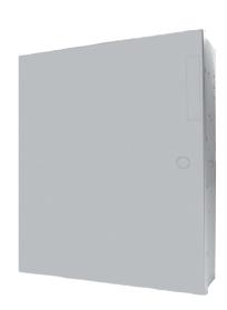
The AE1 is a gray enclosure that accommodates an optional tamper switch for monitoring the door. It is made of 1.0 mm cold-rolled steel and includes a keyed lock. The dimensions are  $35.6 \text{ cm} \times 31.8 \text{ cm} \times 7.6 \text{ cm}$  (14 in. x 12.5 in. x 3 in.).
