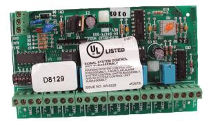
The D8129 Octo-relay Module is suitable for applications requiring Form C relays to operate auxiliary systems or to display fire system status at remote annunciators. Building components such as HVAC, door lock releases, and stairwell pressurization can interface with the D8129 for complete system control and monitoring.
