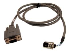
The MAP Serial Cable provides connection between the MAP DE Module and a transmission unit or the GPRS modem (ITS-MAP0008). It consists of a 1.6 m (5.25 ft), gray PVC-sheathed cable with a DB9 male terminal plug at one end and a DB9 female terminal socket at the other end.
