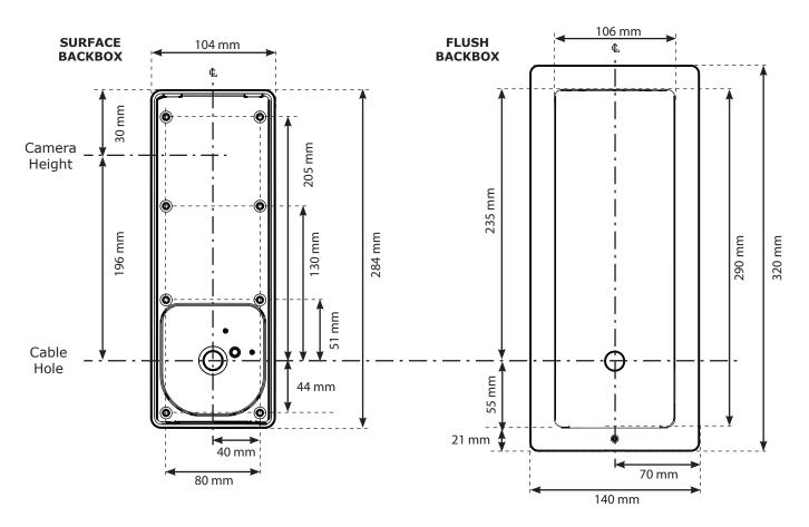
The unit is supplied with the surface mount backbox. A flush mount backbox is also available (PN:337-857). Screws and wall plugs are provided in the fitting kit.
