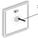
Press and hold the key button and hold any standard key up to the circle on the center of the reader at a maximum distance of 2 cm until the red LED flashes and you hear two short confirmation signals.
