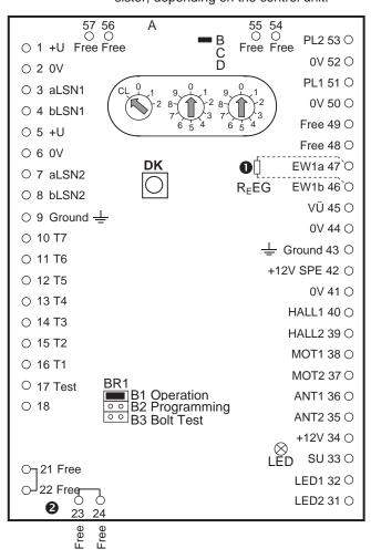
A, B, C or D is equipped with an SMD resistor, depending on the control unit.
