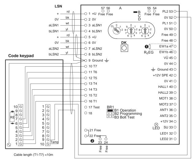
Terminating resistor RESG tamper in code keypad 12K1
